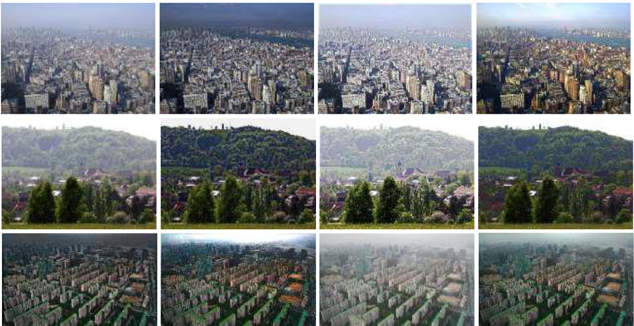
Figure 1. From left to right: the original image, the enhanced image by Tarel [5], Liao [8] and our method.
